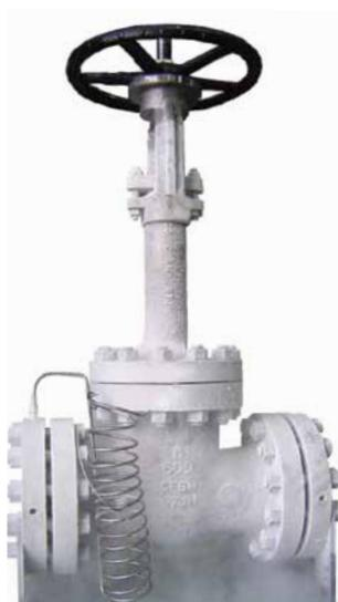
**Extended Bonnet** Bolted or integral vapour space extended bonnet of sufficient length to keep stem packing out of the cold zone and free of ice formation.
